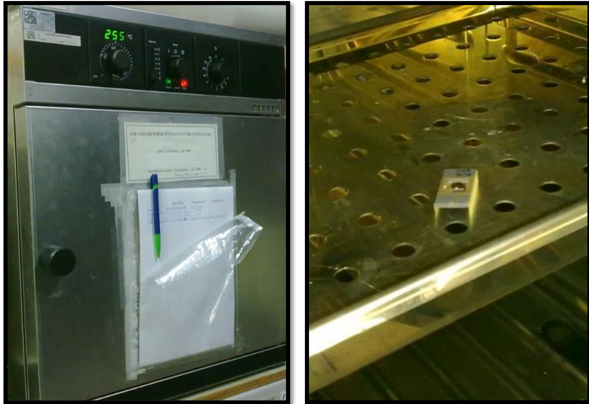
Figure 22 – Memmert heating oven and chip inside oven
